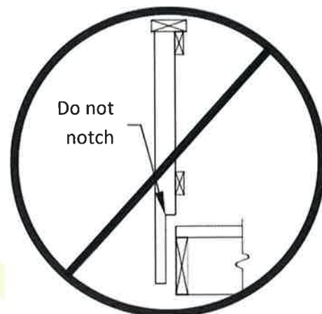
Figure 19. Post Notches Prohibited
